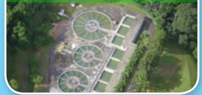
Water & wastewater treatment plants consist of treatment pools, mixers, pH control pools and precipitation pools: requiring different process functions and equipment. The compact ADAM series modules can receive data from the control room, send commands to process simple demands and control the quality. The ADAM series can also be used to monitor pipeline pressure, temperature, flow and leakage when water is transported through the pipelines.
